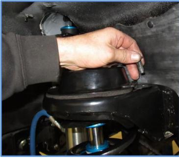
6. Install reservoir bracket. First place the reservoir in the clamp as shown. Then place the spacers in position over the holes for the coil bucket cap where you previously removed the bolts. Then place the reservoir bracket over the spacers and install the supplied M10 X 80mm bolts (CB3731) as shown.
