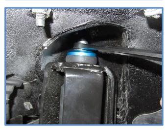
Important Note: The rubber bushings on your King shocks are different from each other. Make sure the taller bushing is on the bottom next to the body of the shock as shown.
