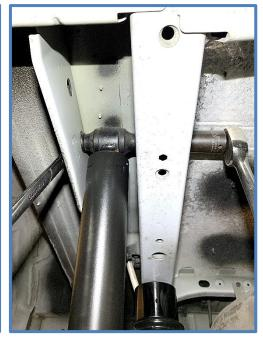
3. Install King Shocks in the factory mounts reusing the factory hardware as shown below. Reservoirs should be facing towards front of vehicle and stickers facing out towards leaf spring. Place shock in the upper mount and install the factory bolt. Place nut on bolt and torque to factory specs.
