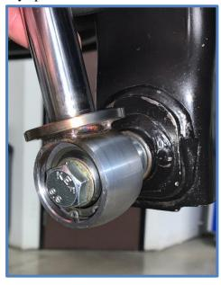
7. Tighten upper nut using a 3/4" wrench.
