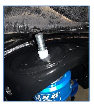
5. Place the upper bushing on the mounting stud followed by the blue retaining washer, 1/2" washer and nut. Apply anti-seize to the threads and thread the nut on finger tight for now to hold the shock in place.
