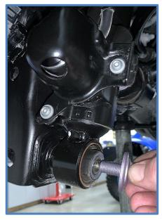
3. Remove the upper mounting nut using a 22mm wrench. You may need to hold the stud with pliers or vise grips to loosen the nut. Remove shocks from vehicle.
