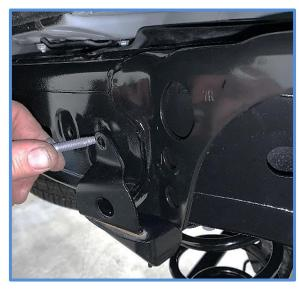
11. Slide the reservoir bracket over the reservoir, then place the bracket over the backing plate as shown below. Install the two short 8mm bolts (CB3825) into the backing plate and install the longer 8mm bolt (CB3824) through the bracket and thread into the existing bump stop hole in frame where you just removed the factory bolt. Tighten all bolts using a 12mm wrench or socket.
