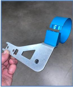
9. Insert the Backing Plate (25049-040) into the rectangular hole in frame with the rounded corners facing towards the front of vehicle. Flip the plate out with thumb as shown below and slide forward to hold in place.
