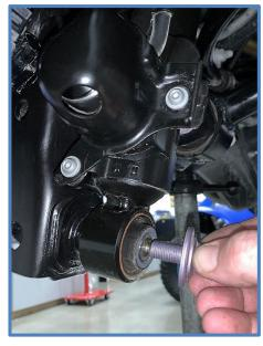
3. Remove the upper mounting nut using a 22mm wrench. You may need to hold the stud with pliers or vise grips to loosen the nut. Remove shocks from vehicle.
