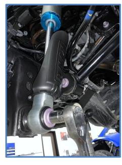
7. Tighten upper nut using a 3/4" wrench.
