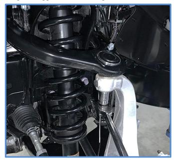
7. Remove the four nuts from the upper mount using a 14mm wrench or socket.
