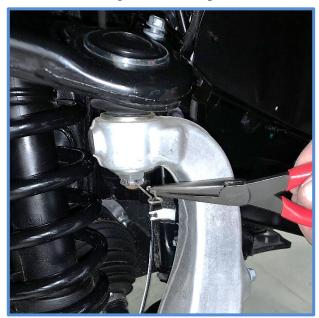
6. Remove upper ball joint nut using a 19mm socket. Separate upper A-arm from spindle.
