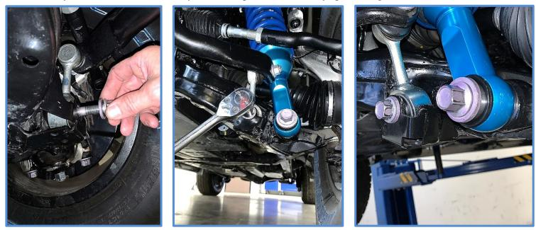
19. You may need to rotate the tie rod boot clamp so that it does not contact the shock. Use pliers to open the clamp and rotate clamp to the top or front side of tie rod.
