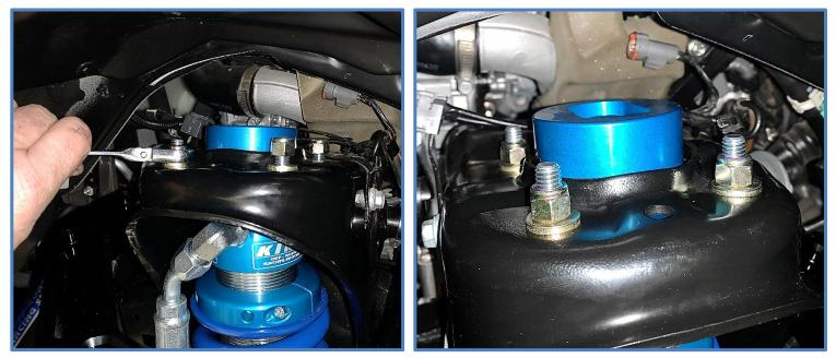
13. Reconnect upper control arm. Tighten castle nut to factory specs and reinstall the pin.
