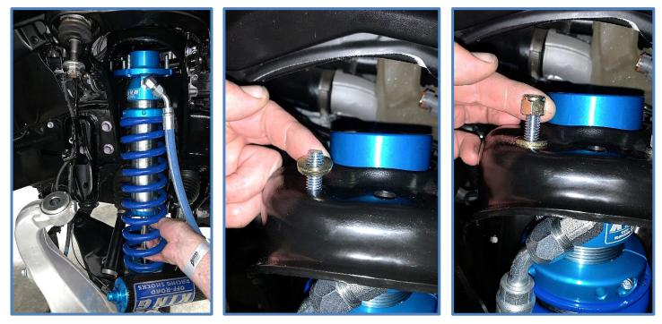
11. Maneuver the rod end onto the lower mounting stud while prying down on the sway bar. Once the rod end is installed, make sure bearing spacers and bushings are properly positioned and install the factory bolt. Tighten the lower bolt to factory specs.
