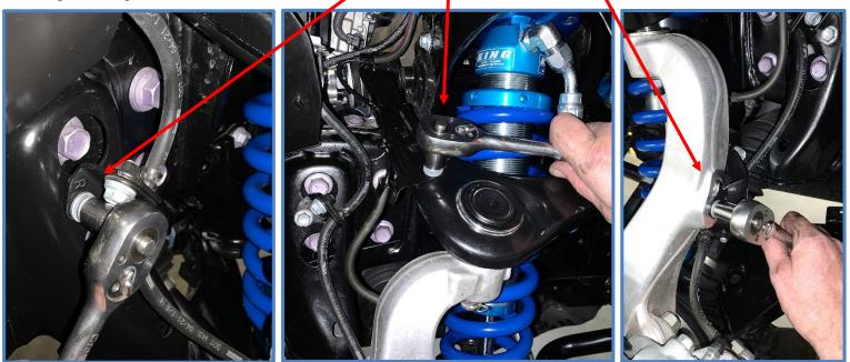
15. <u>Mount Reservoirs</u> – First attach reservoir clamps to the reservoir brackets using the supplied 1/4 x 1/2" BHCS (CB2420). Apply red locktite to the threads and attach clamps to brackets as shown below.
