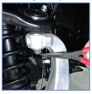
6. Remove upper ball joint nut using a 19mm socket. Separate upper A-arm from knuckle.
