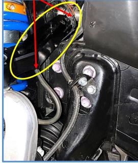
17. Mount Reservoirs – First attach reservoir clamps to the reservoir brackets using the supplied 1/4 x 1/2" BHCS (CB2420). Apply red locktite to the threads and attach clamps to brackets as shown below.
