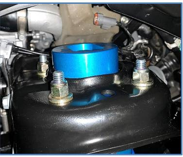
15. This kit requires the use of an aftermarket upper control arm that can accommodate the extra droop that this shock will provide and give adequate clearance for hose between spring and control arm at full droop. It is ultimately up to the installer to check fitment of aftermarket components and address any clearance issues. Install your upper control arms per the instructions that came with your control arm kit.
