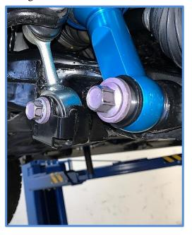
21. You may need to rotate the tie rod boot clamp so that it does not contact the shock. Use pliers to open the clamp and rotate clamp to the top or front side of tie rod.
