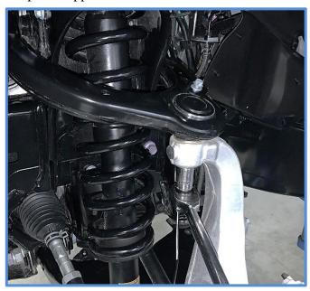
7. Remove the four nuts from the upper mount using a 14mm wrench or socket.
