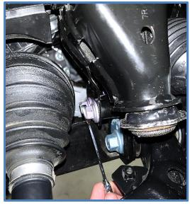
11. <u>Install King Bump Stop Delete Bracket</u> – Be aware the brackets are side specific, see photos for proper orientation. Place bracket in position and install the factory hardware for the lower control arm mount and the factory bolt for underneath the frame. Use the provided M10 button head bolt (CB2450) with M10 washer (CW1802) for the side of frame as shown. Start all bolts by hand then tighten to factory specs.
