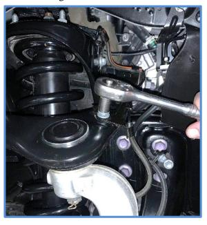
2. Unbolt the ABS/brake line bracket on the frame and knuckle using a 12mm wrench or socket.
