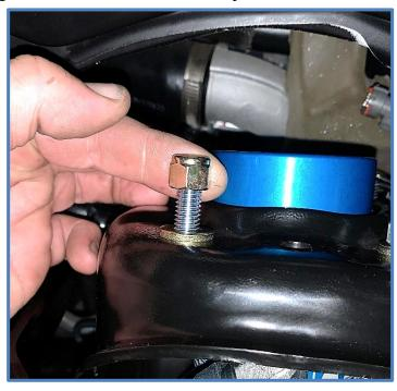
13. Place the thinner bearing spacer with bushing on the lower mounting stud first. Then maneuver the rod end onto the lower mounting stud while prying down on the sway bar. Once the rod end is installed, place the thicker bearing spacer with bushing on the stud followed by the factory bolt. Tighten bolt to factory specs.
