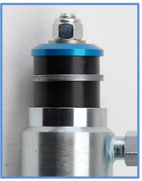
12. Install the 1/4 x 1" SHCS (CB1501) in the reservoir clamp. Adjust reservoir to its final position (See final install pictures for reference) and tighten bolt using a 3/16 Hex Key.
