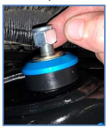
10. Place the rod end on the lower mounting stud with shaft guard facing forward and install the factory bolt. Torque bolts to factory specs.
