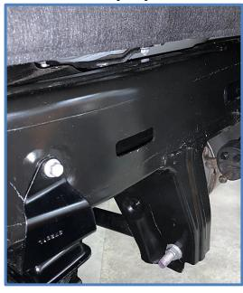
5. Insert the Backing Plate (25049-040) into the rectangular hole in frame with the rounded corners facing towards the front of vehicle. Flip the plate out with thumb as shown below and slide forward to hold in place.
