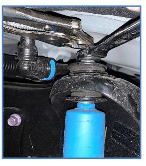
3. Mount Reservoir Brackets – First attach reservoir clamps to the reservoir brackets using the supplied 1/4 x 1/2" BHCS (CB2420). Apply red locktite to the threads and attach clamps to brackets. Tighten screws using a 5/32 Hex Key. Photos below show the left bracket.
