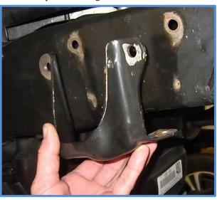
3. Place the bracket in position on the frame and install the 7/16 X 1" bolts (CB4601) with washers (CW1001). It may be necessary on some vehicles to enlarge one or more of the holes in the frame to install hardware. Tighten the lower bolts first using a 5/8 wrench and socket, then tighten the upper bolts.
