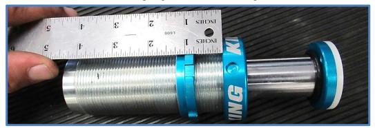
7. Now place the bump stop in the bracket and thread the upper lock ring onto the bumpstop.
