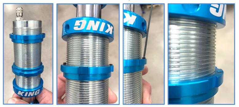
10. Thread lower stop nut all the way down as shown below.
