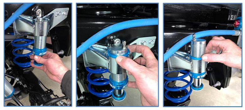
12. Make sure the set screws are backed out before tightening the upper nut. Then tighten upper stop nut using a hammer and screwdriver or punch. Tighten upper nut then tighten set screws.
