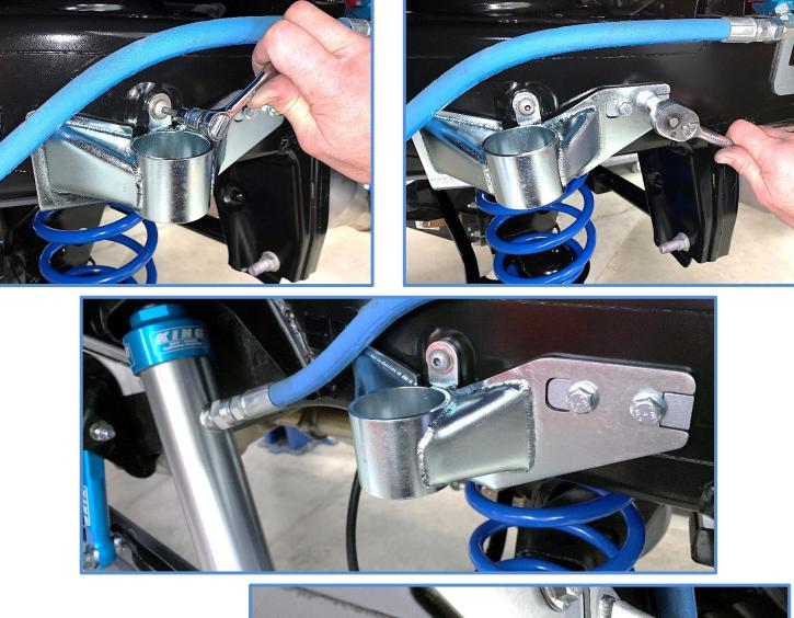
Make sure bracket is sitting flat against the side of frame and bottom of frame.
