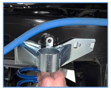
5. Use the supplied 8mm flanged bolts (CB3825) for the backing plate. Thread bolts in by hand to hold in place for now. Do not tighten any bolts until all bolts have been installed and threaded in by hand.
