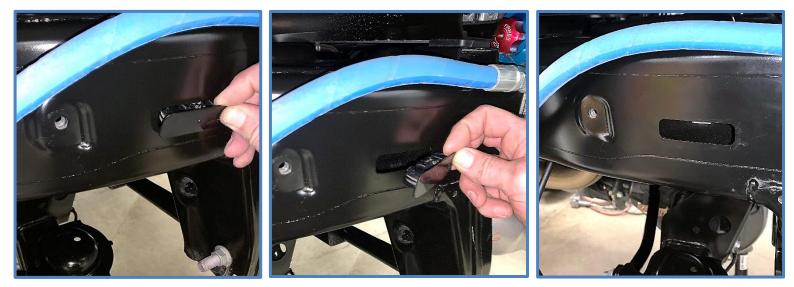
3. Insert the Backing Plate (25049-040) into the rectangular hole in frame with the rounded corners facing towards the front of vehicle. Flip the plate out with thumb as shown below and slide forward to hold in place. (Use a magnet or thread a bolt into plate to help pull backing plate out if you are having trouble.)
