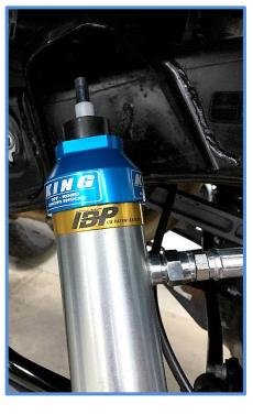
5. Place the upper bushing on the mounting stud followed by the blue retaining washer, 1/2" washer and nut. Apply anti-seize to the threads and thread the nut on finger tight for now to hold the shock in place.
