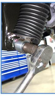
7. Tighten upper nut using a 3/4" wrench.
