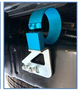
11. Slide the reservoir into the clamp as shown below.
