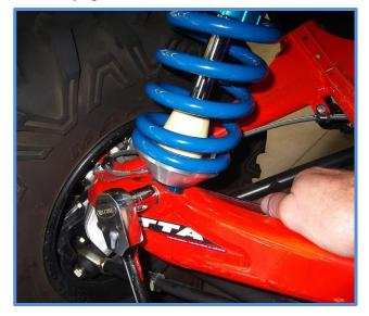
Double check your install, make sure the shocks are mounted properly and all hardware is tight. Recheck the hardware after 50 miles and periodically after that as part of routine maintenance.
