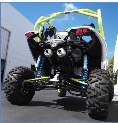
Double check your install, make sure the shocks are mounted properly and all hardware is tight. Recheck the hardware after 50 miles and periodically after that as part of routine maintenance.
