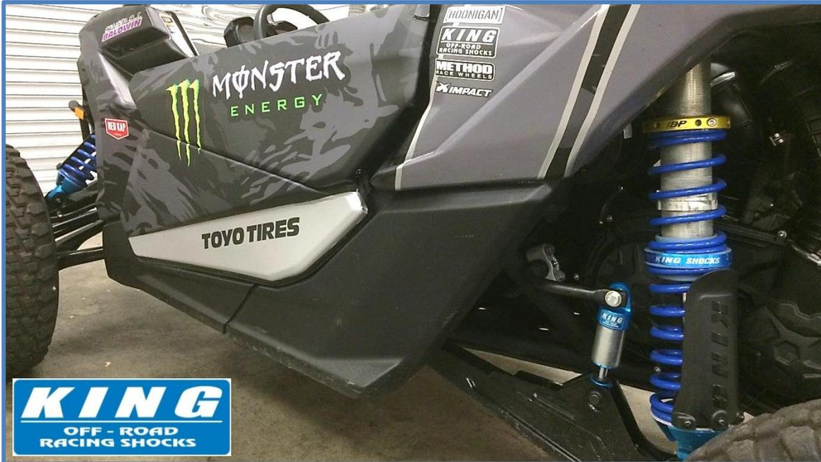
1. Remove stock sway bar link by first removing the upper nuts on both sides of the vehicle using an 18mm socket on the nut and a 21mm wrench to hold the ball joint from turning. Next remove the lower bolts using an 18mm wrench and socket. Save all factory hardware, you will reuse it to mount the sway bar shocks.
