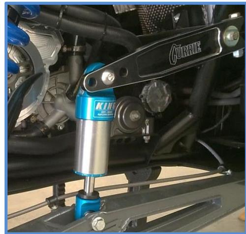
**Double check your install, make sure the shocks are mounted properly and all hardware is tight. Recheck the hardware after 50 miles and periodically after that as part of routine maintenance.**
