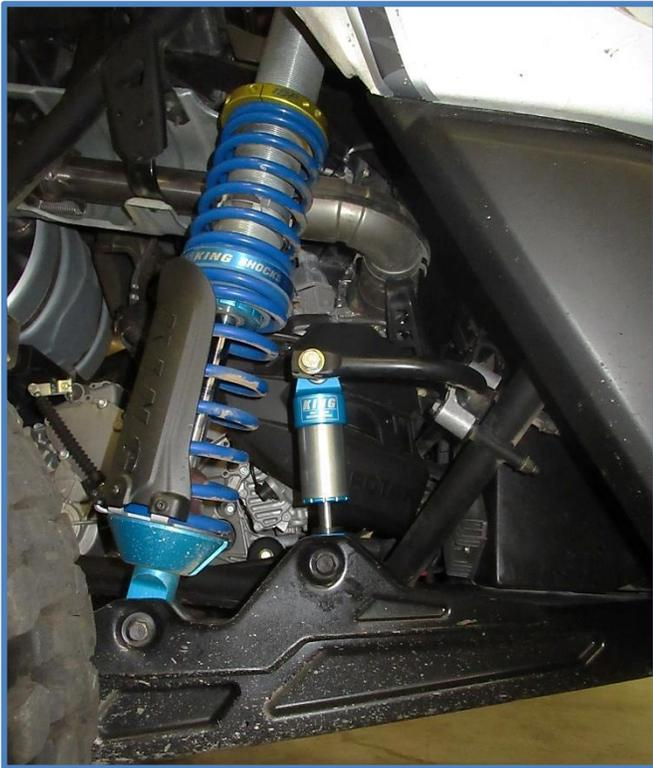
Can-am X3's with AFTERMARKET sway bar or AFTERMARKET trailing arm may require modifications to spacers to accommodate a larger bolt or different mounting width's.
