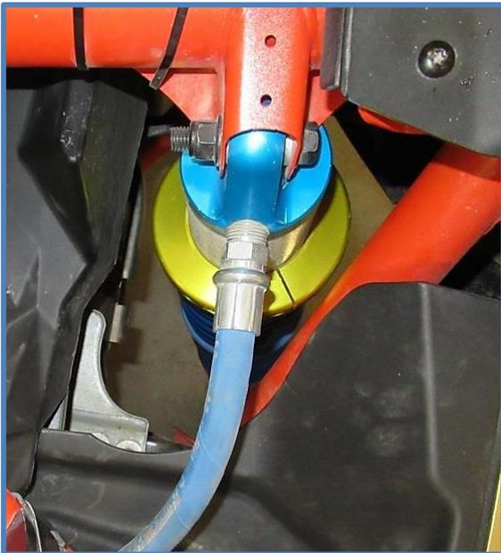
5. Place the rod end in the lower mount and install the lower mounting bolt and nut. Tighten all bolts to factory specs.
