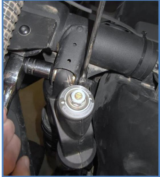
4. Install King Shocks using the factory hardware.
