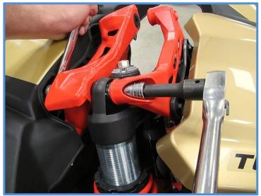
King Shocks should be mounted with reservoirs facing outward for easier access to compression adjusters and Schrader valve. This also allows more air flow to the reservoirs for better heat dissipation and maximum performance.
