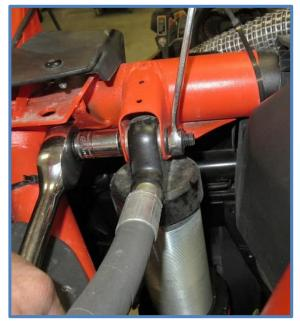
4. Install King Shocks using the factory hardware. Place shock in position on the vehicle and install the upper mounting bolt and nut.
