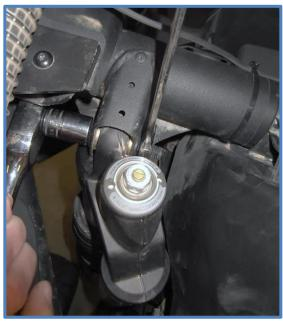
5. Place the rod end in the lower mount and install the lower mounting bolt and nut. Tighten all bolts to factory specs.
