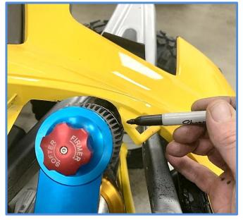
Continue trimming as you lower the vehicle to create a nice cut around the reservoir.
