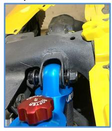
10. Place rod end in lower mount and install factory bolt. Torque upper and lower bolts to factory specs.
