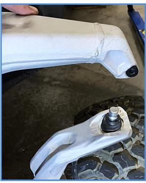
7. Fender trimming is required to mount front shocks. Installing shocks without springs and lowering the vehicle as you are trimming is the best way to make accurate cuts, trim plastic in stages as you lower the vehicle to the fully compressed position. See photos below and on the next page for trimming example.
