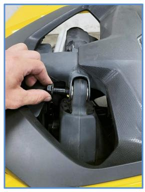
5. Remove the pinch bolt on the upper control arm using a 15mm wrench and socket.
