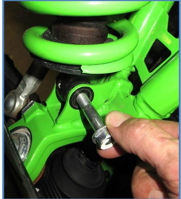
3. Unbolt the upper mount using a 17mm wrench/socket. Remove bolt and save hardware for reuse. Remove shock from vehicle.
