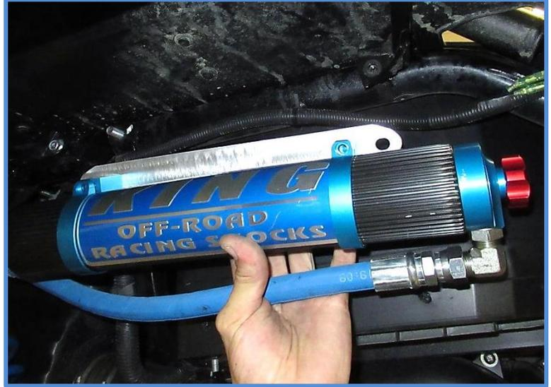
7. Now place the reservoir bracket over the front bolt and between the rear support brackets, line up holes in rear and reinstall the bolt. Install nut on front bolt and tighten to factory specs.
