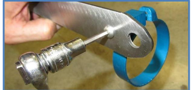
Photos shows left side with large hole in front and the smaller slotted hole to the rear with the clamp hanging down. Right side will be a mirror image of this.
