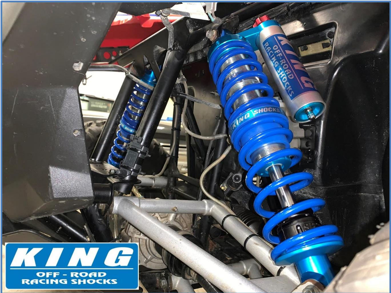
**Double check your install, make sure the shocks are mounted properly and all hardware is tight. Recheck the hardware after 50 miles and periodically after that as part of routine maintenance.**
