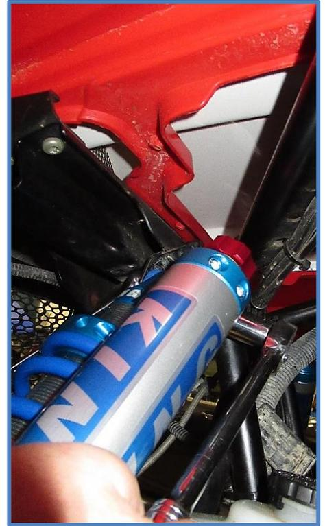
3. Place the rod end in the lower mount, install the factory bolt and tighten to factory specs.
