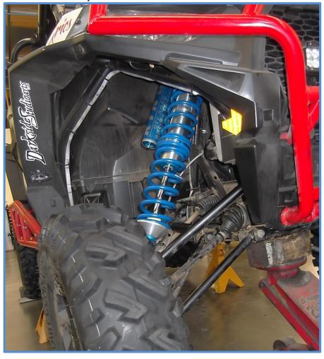
Double check your install, make sure the shocks are mounted properly and all hardware is tight. Recheck the hardware after 50 miles and periodically after that as part of routine maintenance.
