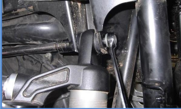
2. Install King Shocks using the factory hardware. Be aware that the shocks are side specific and need to get installed with the reservoirs towards the front of the vehicle. See step three for special instructions for mounting rear shocks.
