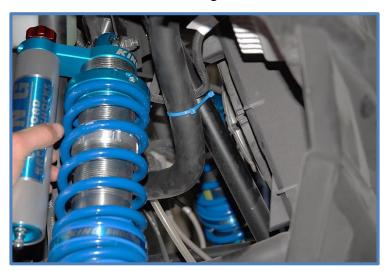
Double check your install, make sure the shocks are mounted properly and all hardware is tight. Recheck the hardware after 50 miles and periodically after that as part of routine maintenance.
