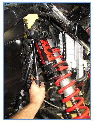
4. Install King Shocks using the factory hardware. Be aware the shocks are side specific. Place the shock in position with the reservoir towards the rear of the vehicle and install the factory bolt in the upper mount first.
