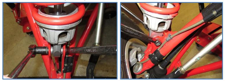
3. Remove the upper mounting bolt using a 15mm wrench and socket then remove shock from vehicle.
