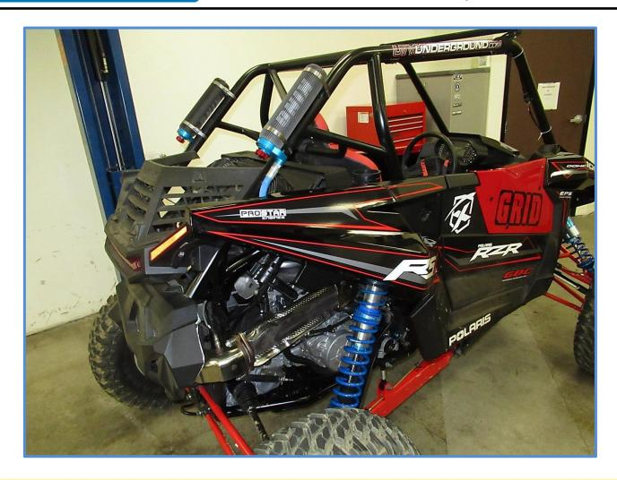
Double check your install, make sure the shocks are mounted properly and all hardware is tight. Recheck the hardware after 50 miles and periodically after that as part of routine maintenance.
