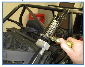
3. Remove the lower mounting bolt using an 18mm wrench and socket.
