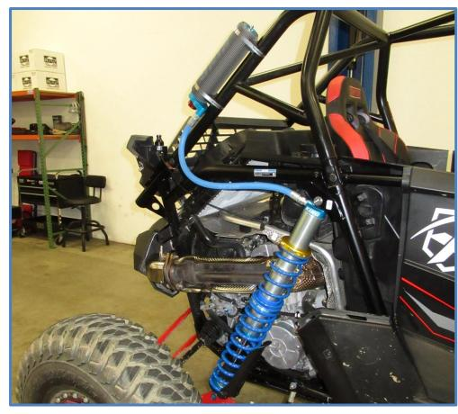
Depending on how you route the hose and where you mount the reservoir you may need to trim the side panels for hose clearance before finishing the install.
