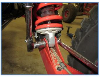
4. Remove the upper bolt using an 18mm wrench and socket and remove shock from vehicle.
