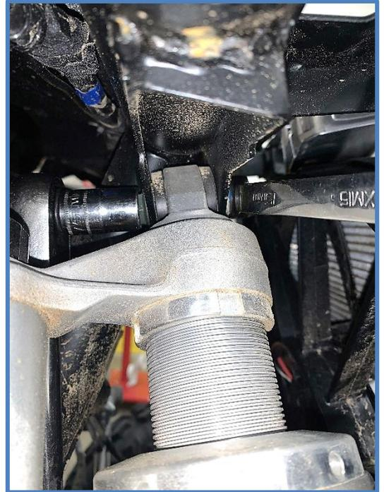
4. Install King Shocks using the factory hardware. Be aware the shocks are side specific. Place the shock in the upper mount with the reservoir towards the rear of the vehicle and install the factory bolt and nut.
