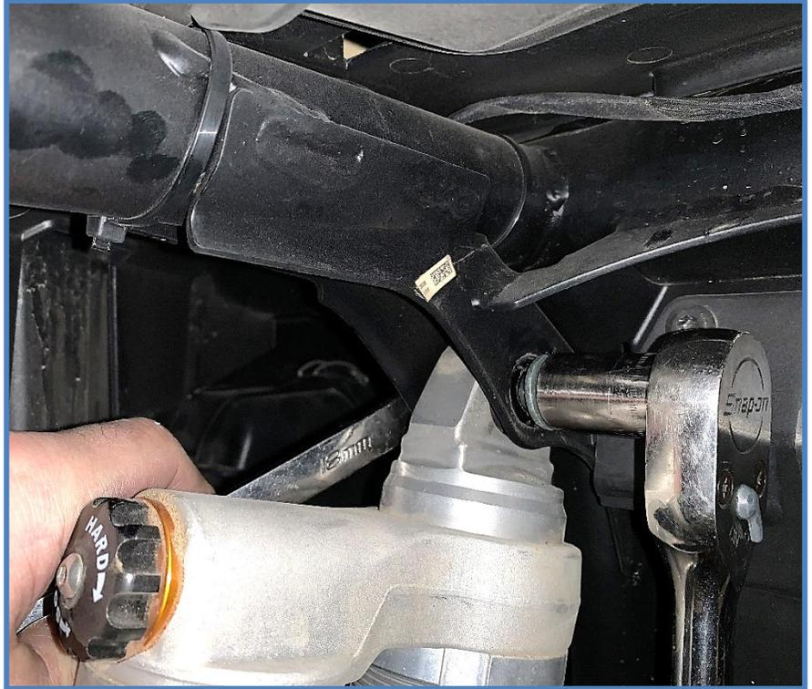
4. Install King Shocks using the factory hardware. Be aware the shocks are side specific. Place the shock in the upper mount with the reservoir facing out towards the tire and back towards the rear of the vehicle. Install the factory bolt and nut in the upper mount.
