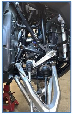
Important Note: Before installing your King Shocks, double check to make sure the clevis is positioned properly. One side of the clevis has a large radius for axle clearance. Make sure the large radius is towards the axle, opposite of the reservoir.
