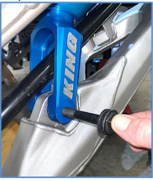
8. Torque upper and lower mounting bolts to factory specs. Repeat steps on opposite side of vehicle before reconnecting sway bar links.
