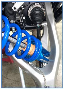
Move top of shock into fender behind the upper mount.
