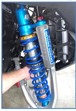
Lift shock up until you can get the clevis over the axle. Rotate clevis over axle as shown below.
