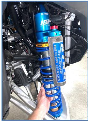
6. Place the factory bolt in the upper mount and thread the nut on for now.
