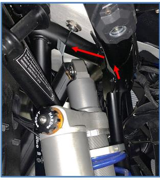
Lift shock up until you can get the clevis over the axle. Rotate clevis to the front side of axle as shown below.
