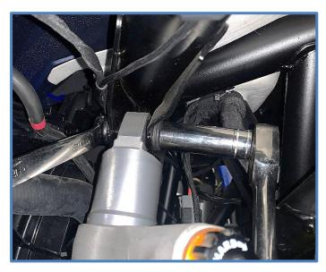
3. Disconnect the sway bar by removing the upper bolts from the sway bar links using an 18mm wrench and socket.
