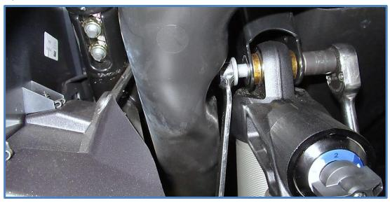
3. Install King Shocks. Be aware the shocks are side specific; make sure the longer bearing spacer on the lower rod end is facing in towards the frame. Place the shock in the mounts on the vehicle and install the factory upper bolt and nut.
