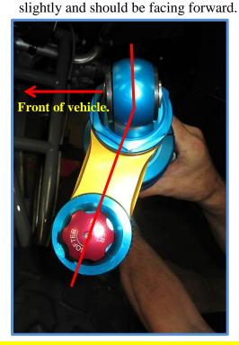
3. Remove the upper bolt using a 15mm wrench or socket on the bolt head and an 18mm wrench or socket on the nut. On the right side you will have to use a wrench on the nut.
