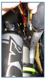
5. On the right side of the vehicle you may need to flip or rotate the hose clamp so it doesn't interfere with shock.
