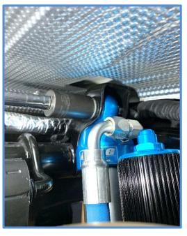
8. <u>Right Side</u> – Place the rod end in the lower mount with the long spacer towards the frame. Install the factory bolt and torque to factory specs.
