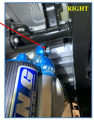
4. <u>Left Side</u> – Place the shock in the upper mount with the long spacer towards the frame. Install the factory bolt in the upper mount and torque to factory specs.
