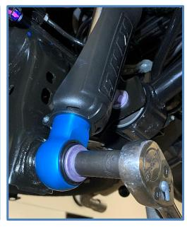
7. Tighten upper nut using a 3/4" wrench.
