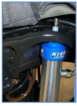
5. Place the upper bushing on the mounting stud followed by the blue retaining washer, 1/2" washer and nut. Apply anti-seize to the threads and thread the nut on finger tight for now to hold the shock in place.
