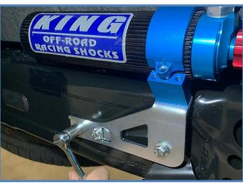
13. Install the 1/4 x 1" SHCS (CB1501). Adjust reservoir to its final position and tighten bolt using a 3/16 Hex Key.
