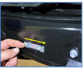
11. Remove the bolt from the bump stop bracket on the outside of frame using a 12mm socket.
