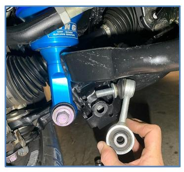
4. <u>Install King Sway Bar Links</u> - Make sure to install links with spacers facing the correct way. Follow the install guide for proper orientation. Failure to install links as shown may cause damage to product and/or vehicle.
