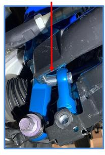
6. Install the provided 14mm X 80mm Bolt (CB3836) with washer (CW1805) through the sway bar link and into the sway bar so that the longer spacer is facing the sway bar and the nut will be on the outside of the sway bar. Install a washer and nut (CN3007) and thread nut on finger tight for now.
