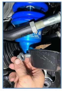
3. Remove factory sway bar links from both sides of vehicle.
