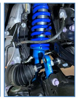
3. Use the supplied M16 bolt (CB3839) with washers (CW1803) and nuts (CN3003) to attach the sway bar link to the sway bar. Place one of the washers on the bolt followed by the short spacer and install through the sway bar link.
