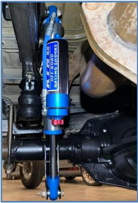
**DOUBLE CHECK ALL HARDWARE:** Make sure everything is installed correctly and all hardware is tight. Recheck all hardware after 100 miles and periodically after that as part of routine maintenance.
