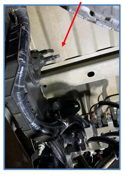
3. When installing King Shocks, make sure the longer spacer is towards the frame as shown below.
