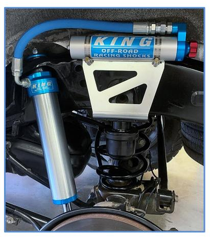
Double check all hardware, install tires and lower the vehicle. Check all hardware and lug nuts after 100 miles and periodically after that as part of routine maintenance.
