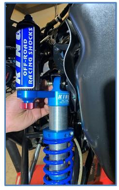
3. Place rod end in the lower mount, install the factory bolt and check clearance between spring and the upper control arm. It may be necessary to grind the upper control arm to make sure there is adequate clearance.
