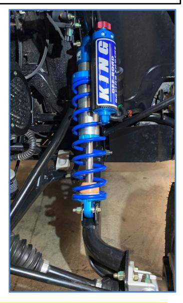
Double check your install, make sure the shocks are mounted properly and all hardware is tight. Recheck the hardware after 50 miles and periodically after that as part of routine maintenance.
