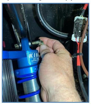
3. Place the rod end in the lower mount, install the factory bolt and tighten to factory specs.
