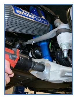
15. Tighten the upper mounting nuts using a 9/16 wrench or socket and torque to 35 ft/lbs. Do not overtighten.
