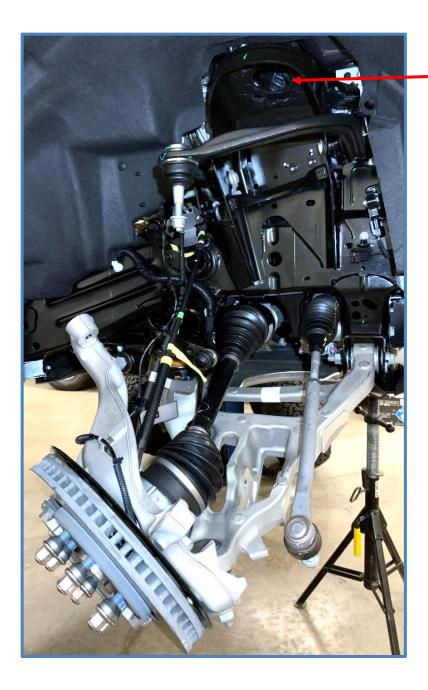
On the right side of the vehicle there is a hose clipped to the body above the shock mount. You may need to unclip the hose to fit the shock. Unclip the hose and move out of the way. Secure hose with zip ties in other location to keep from getting damaged.
