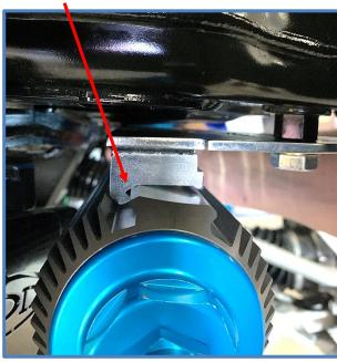
21. Install the retaining clips with the provided 1/4-20 X 1.75 SHCS (CB1508). Make sure the retaining clip engages in the groove on the reservoir.
