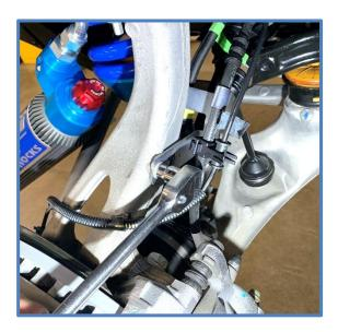
17. <u>Reservoir Mounting</u> – Be aware reservoir brackets are side specific. Photos below show the right side. Place reservoir bracket on the nuts on the front cross member as shown.
