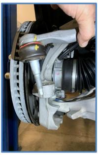
5. Remove nut from the upper control arm ball joint using an 18mm wrench or socket. You may need to use an 8mm wrench to hold the stud. Separate ball joint from knuckle.
