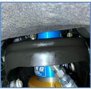
11. Install factory bolt in lower mount. Place flag nut in position so the handle is in the locating hole and thread bolt into nut to hold in place for now.
