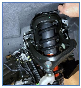
7. Remove the lower mounting bolt using a 27mm socket, you may need a breaker bar to loosen the bolt.
