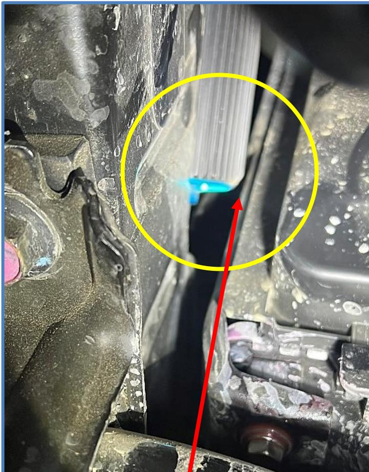
Make sure there is adequate clearance between the end of reservoir and the edge of the radiator. You should be able to easily get your fingers between the reservoir and the radiator.
