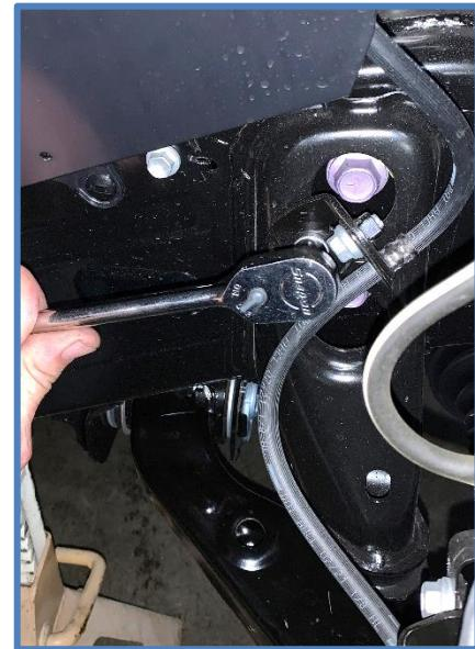
2. Remove pin from upper ball joint, loosen nut with a 19mm socket. Separate upper A-arm from spindle.
