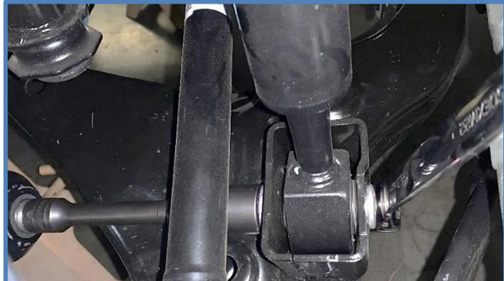
5. Remove upper mounting nuts using a 14mm wrench or socket, then remove shocks from vehicle.
