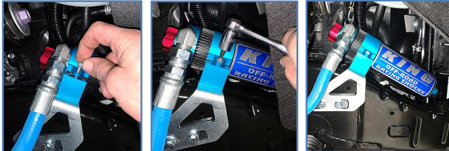
17. **Install Sway Bar Spacer** – Remove the two bolts holding the sway bar to the frame using a 17mm socket. Do one side at a time...
