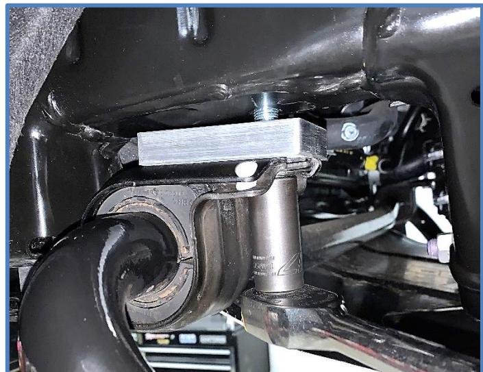
20. Install Skid Plate Spacers – First remove the two bolts in the front of skid plate using a 12mm socket.
