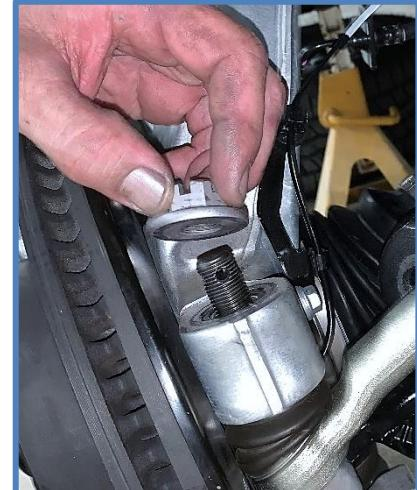
4. Remove lower shock mounting bolt using a 22mm wrench and socket.
