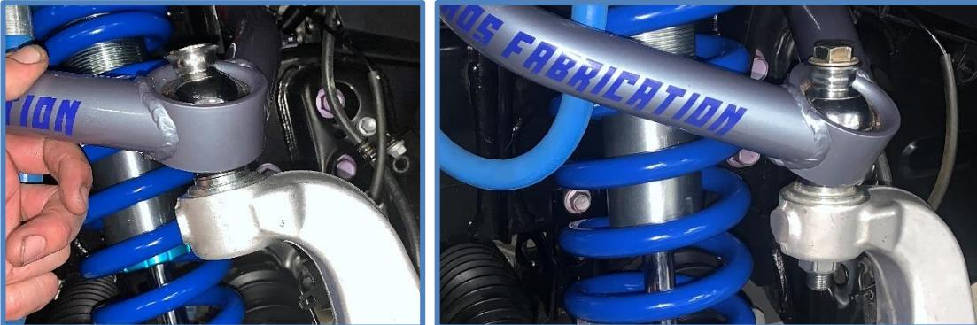
12. Reconnect the brake and ABS lines to the frame, upper control arm and knuckle. Tighten bolts to factory specs using a 12mm socket.
