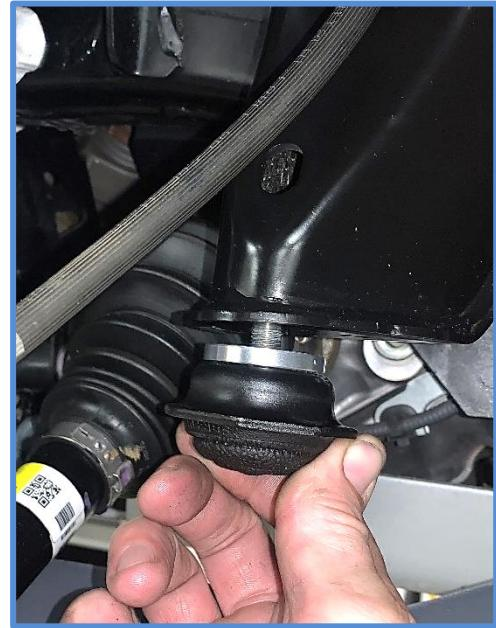
7. **Install King Shocks** – Be aware shocks are side specific. The hose and reservoir will go towards front of vehicle. Place shock in position on the vehicle by first maneuvering top of shock into upper mount. Then pry down on lower control arm and place rod end in the lower mount. Photos below show left side.
