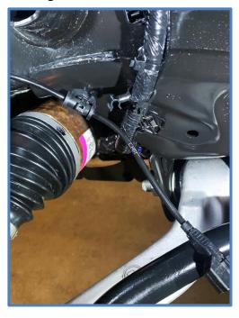
3. Use a pry tool to remove the cable clips from the frame. Unclip wire from frame.
