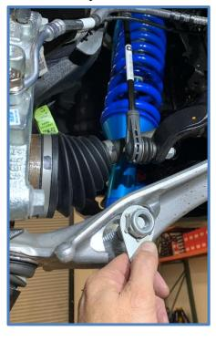
10. Reconnect upper control arm, tighten nut and torque to factory specs. (You may need an 8mm wrench to hold the stud)
