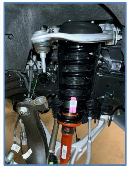
5. Remove the lower mounting bolt using a 27mm socket, you may need a breaker bar to loosen the bolt. (Note: You can leave bolt inserted enough to hold shock in place while removing upper nuts in next step.)
