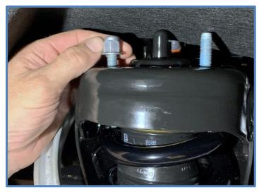
7. Remove shocks from vehicle – Maneuver the bottom of the shock down through the lower control arm until you can tilt the top of the shock out of the upper mount, then pull the shock out of the lower mount and remove shock from vehicle.
