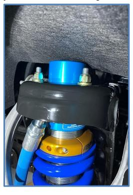
12. Tighten lower mounting bolts and torque to factory specs.
