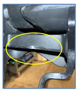
Grind the corner of the bend on the inside of the shock mount (above the studs for the rock guard) as shown below. When you are done modifying the lower mount paint any bare metal to protect from rusting.
