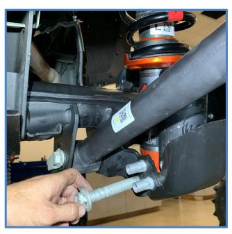
3. Remove rock guard – Use an 18mm socket to remove the two long nuts and remove the rock guard.
