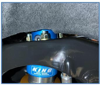
9. Reinstall the rock guard on the lower mount, tighten nuts and torque to factory specs.
