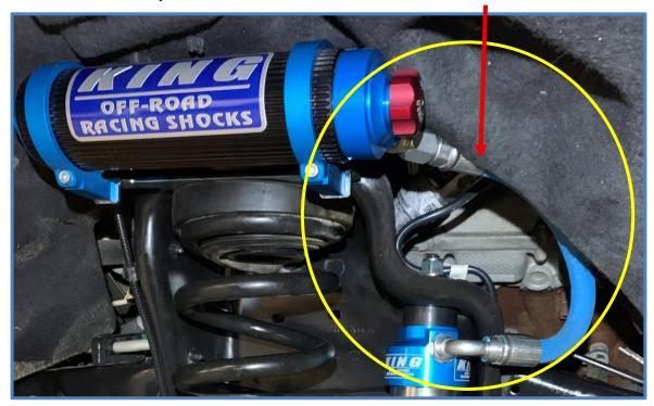
6. Place the upper bushing on the mounting stud followed by the blue retaining washer, 1/2" washer and nut. Apply anti-seize to the threads and thread the nut on finger tight for now to hold the shock in place.
