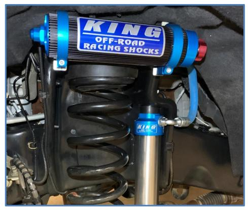
For those installing shocks 25001-432 on a vehicle with an aftermarket lift or leveling kit – Make sure the springs are not loose when the shocks are at full extension. Make sure brake/ABS lines, diff breather, etc. are not too tight when shocks are at full extension.
