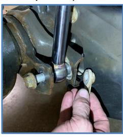
For those installing shocks 25001-432 on a vehicle with an aftermarket lift or leveling kit – Make sure the springs are not loose when the shocks are at full extension. Make sure brake/ABS lines, diff breather, etc. are not too tight when shocks are at full extension.
