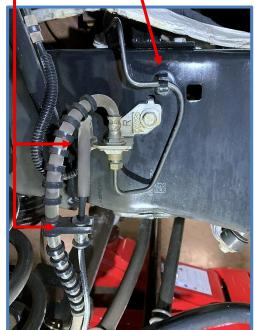
Make sure the brake/ABS lines are not too tight when shocks are at full extension.
