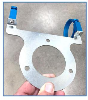
4. <u>Lower the front axle until the springs are loose</u> – You will be mounting the reservoir bracket between the rubber spring isolator and the upper mount. Keep lowering axle until you can slide the reservoir bracket into the upper mount. After reservoir bracket is in position, jack the axle up slightly so the springs can't fall out but leave the spring lowered for now. You need the reservoir bracket to be loose so you can install the reservoir in the next step...
