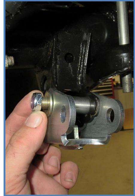
5. Now tighten the 1/2 X 1" bolt on the back side of the bracket using a 3/4 socket, make sure the bracket pulls in tight to the existing mount.
