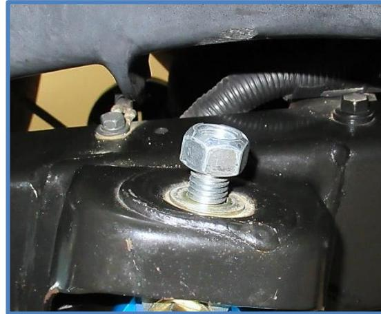
7. Place the rod end in the lower mount and install the 1/2 X 2-3/4" bolt (CB4730) with washer (CW1702). Be aware that these shocks have offset bearing spacers, the longer spacers should be towards the frame which offsets the shock out towards the wheel, this is to provide clearance between the shock and the leaf spring. Make sure the longer spacers are towards the frame. Install the washer (CW1702) and thin nylock nut (CN2800) and tighten both shock mount bolts to 90 ft-lbs.
