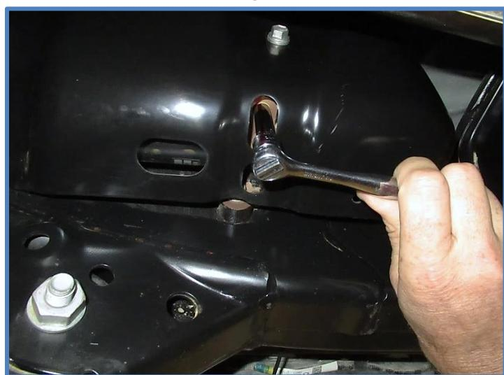
**Warning:** If you unscrew the valves more than three full turns air can get into the KDSS system. If this happens, the vehicle will need to have the hydraulic system serviced by a Toyota dealer.
