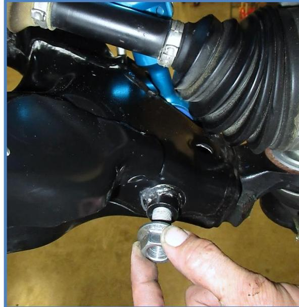
12. Install your upper control arms as per the instructions that came with your control arms. Reconnect tie rod and tighten to factory specs, be sure to reinstall cotter pin. Reconnect the brake and ABS brackets. Now reinstall the sway bar links and tighten bolts to factory specs.
