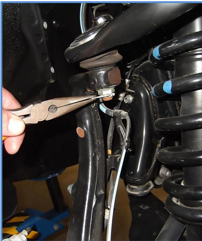
6. Remove upper ball joint nut using a 19mm socket. Separate upper A-arm from spindle.
