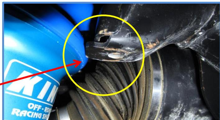
13. **Installing reservoir brackets:** Remove the two bolts from the frame using a 12mm wrench or socket.
