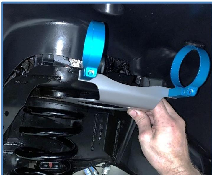
7. Place the reservoir brackets in position on the rubber isolators so the hole for the locating pin lines up. Jack the axle up slowly while checking both sides to make sure the coil is seating properly. Make adjustments as necessary and continue jacking the axle up until the coil begins to compress.
