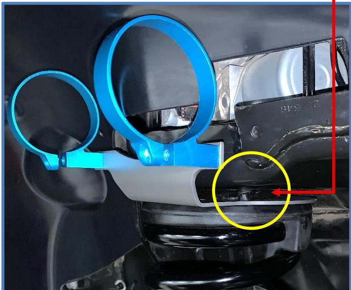
8. **Install King Shocks** - Shocks are side specific, be sure you are installing shocks on the proper side. (See final install picture for reference). Start by removing the nut, washer, anodized blue retainer and upper rubber bushing from the upper mounting stud. Make sure the taller bushing is on the bottom of the stud.
