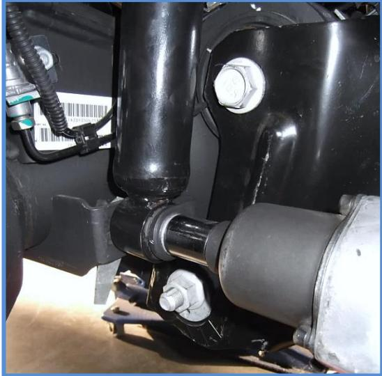
4. Now with both front shocks removed you can lower the front axle until the springs are loose. You will be mounting the reservoir bracket between the rubber spring isolator and the upper spring mount.
