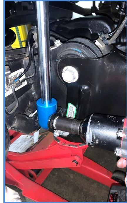
12. Lift axle up so the shock is tight against the upper mount, then tighten the upper mounting nut using a 3/4" wrench per the instructions below.
