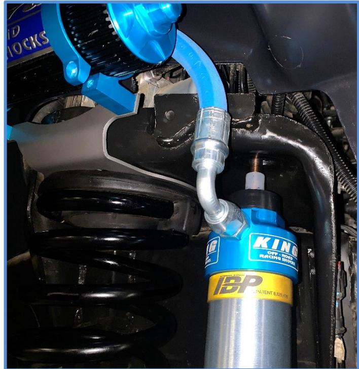
10. Place the upper bushing on the mounting stud followed by the blue retaining washer, 1/2" washer and nut. Apply anti-seize to the threads and thread the nut on finger tight for now to hold the shock in place.
