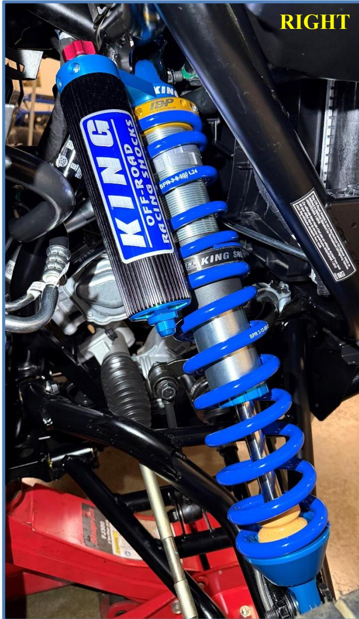
**Double check your install, make sure the shocks are mounted properly and all hardware is tight. Recheck the hardware after 50 miles and periodically after that as part of routine maintenance.**
