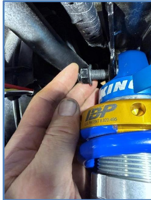
5. Place rod end in the lower mount and install the factory hardware. Tighten upper and lower mounting bolts and torque to factory specs.
